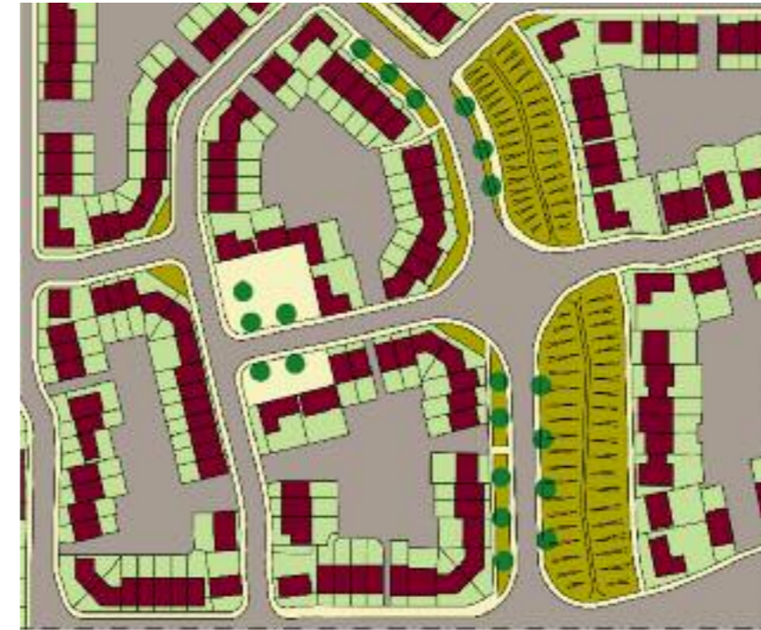
Scheme A - Typical rear parking court layout
