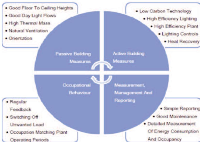
Figure 1: Typical characteristics of a low carbon building (Source: Verdantix and Low Carbon Workplace Partnership, 2011)
