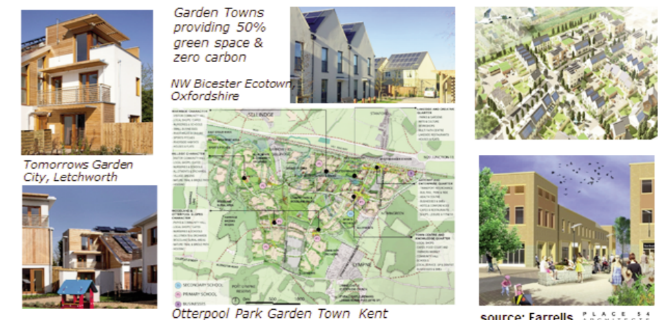
Garden Towns: pop 10,000, area 7km2; block density 250 hrh, 50 homes/ha; district density 15 -20 homes/ha
